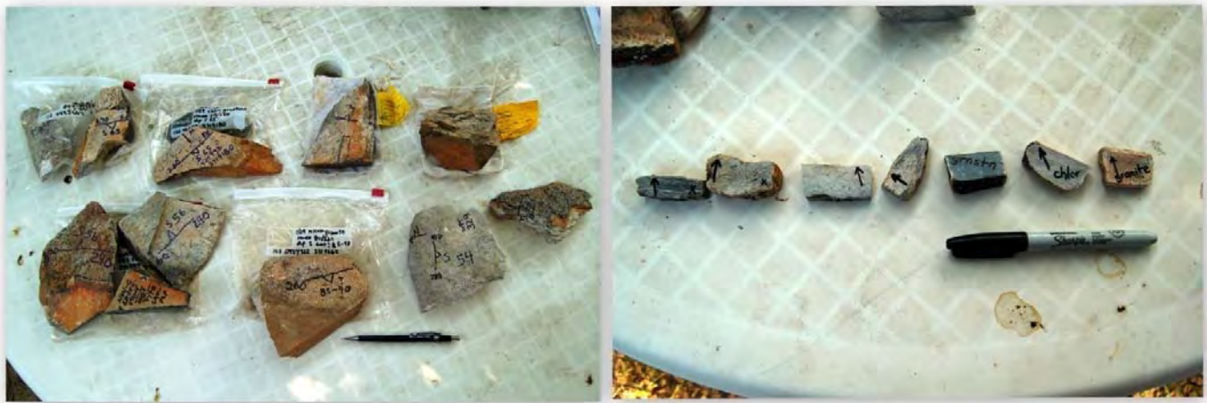
Figure 12. Samples and preliminary cuts prior to thin-sectioning
