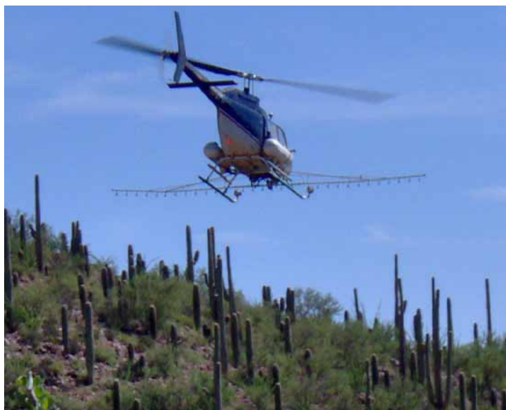
Helicopter with boom sprayer. (US Forest Service)
