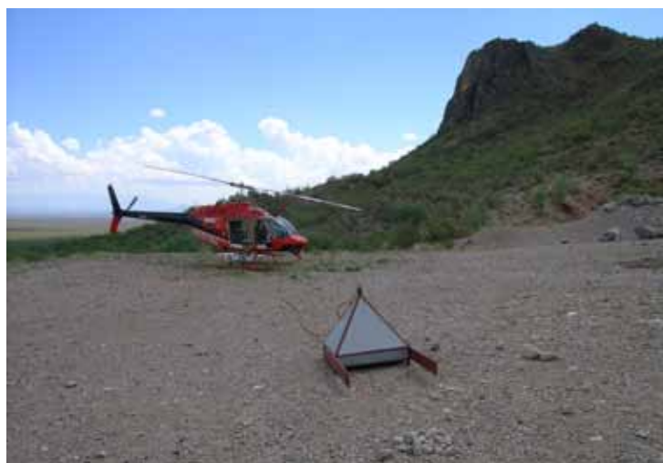
“Pyramid housing” nozzle assembly (US Forest Service)
