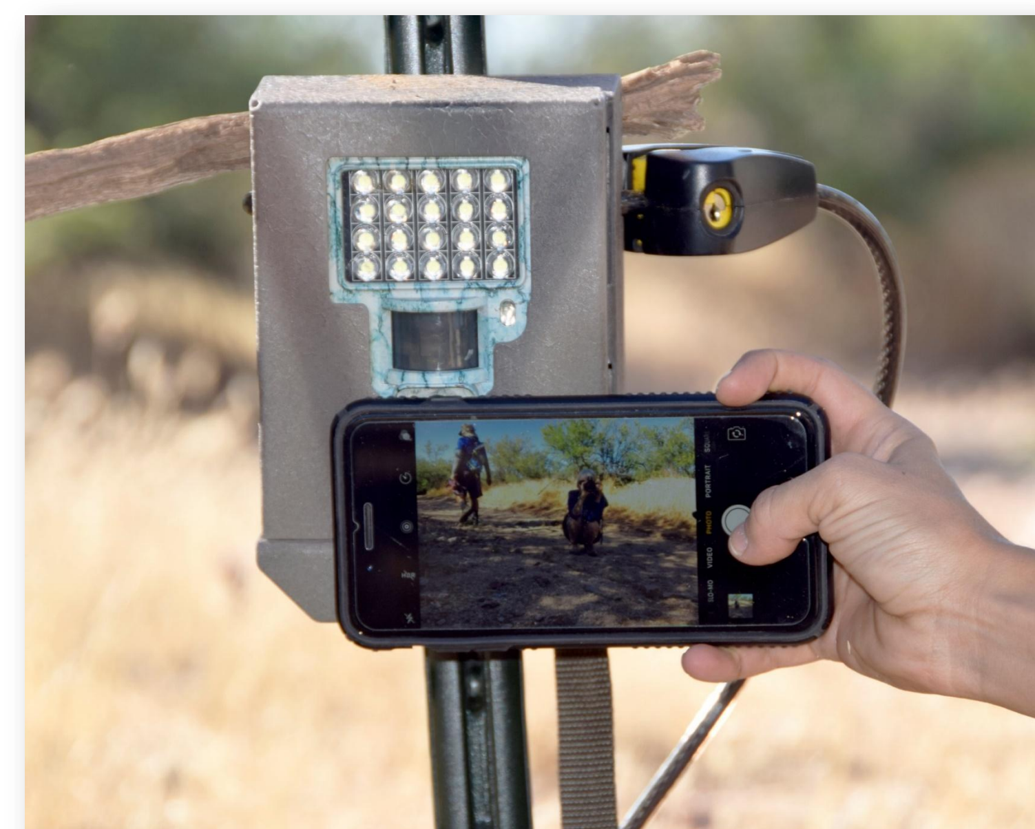
Fig 5. Checking camera field of view with cell phone. Photo: D. Langenfeld
